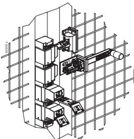
For applications with Category 4, Performance Level e, SAFEMASTER STS units can also be equipped with 2 actuators.
