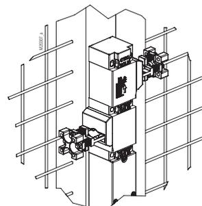
SAFEMASTER STS units with double actuators can be used to monitor 2 adjacent accesses.
