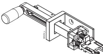
The CS actuator is particularly suitable for harsh and dirty ambient conditions. In addition, the CS actuator is designed for applications with high shear and tensile forces, so that overload breaks can be largely excluded.
