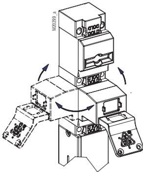
The modular design and the plug-in keys allow a variable alignment of the modules. Keys and actuators can therefore also be operated from the side.
