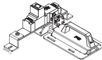
The CW bolt moves under the mounted unit, making the slider suitable for securing hinged doors with both left and right stop. It is designed in such a way that shear forces cannot act directly on the STS unit. It is particularly suitable for applications, where high forces can act on the STS units, e.g. in double swing doors.
