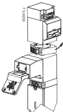
Units can be mounted simple and easily via ring locks (bayonet ring).
