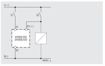
Control with parallel connected load
