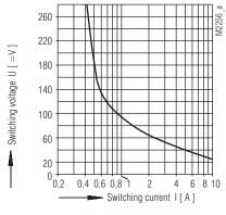
safe braking, no continuous arcing max. 1000 switching cycles / h contact spacing min. 0,6mm
