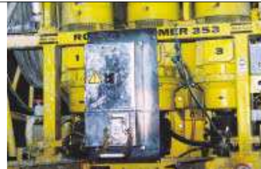
A Cavotec panel mounted on an Atlas Copco shotcrete machine.
