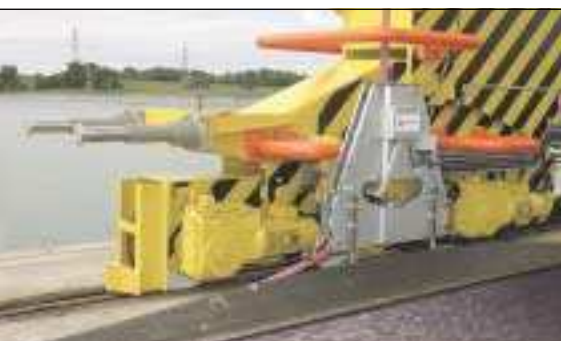
The flexible belt, together with the specially designed belt-lifting unit, ensures a smooth and trouble-free travel of the crane.
