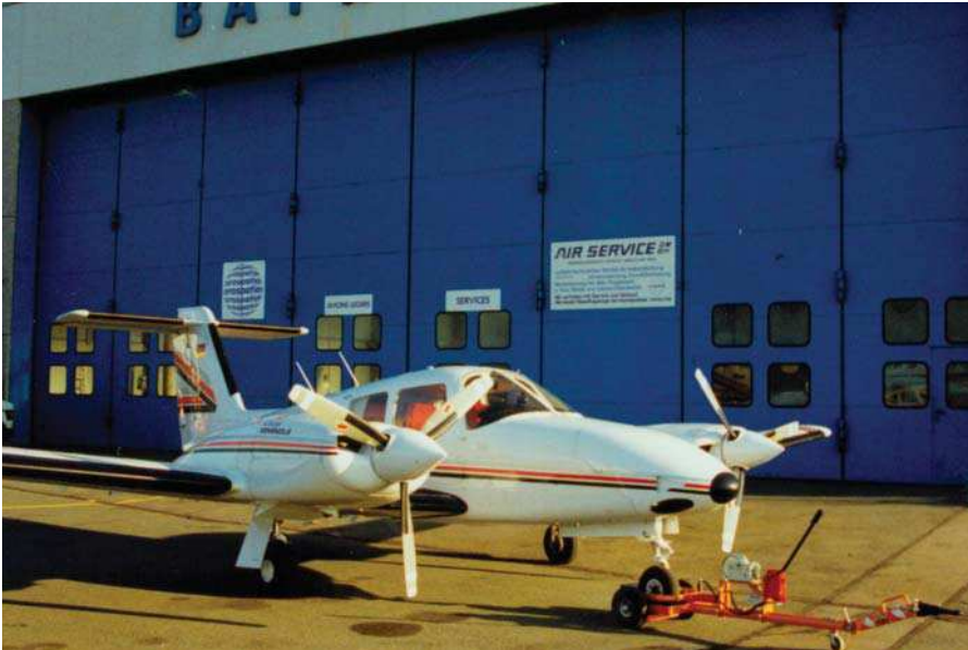
This towbar is specially designed for towing small aircraft with upto 2000kg nose wheel weight.
