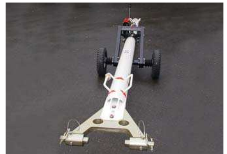
Towbar fitted with the adapter-head for IL62 aircraft.
