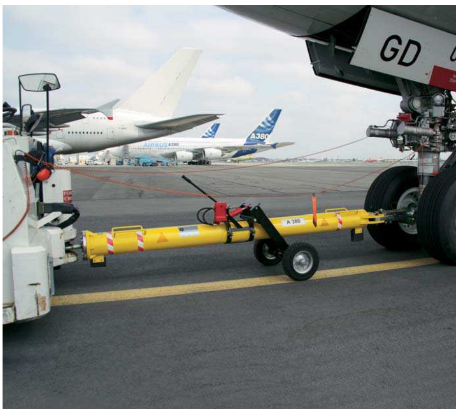
A Cavotec Fladung towbar in action.
