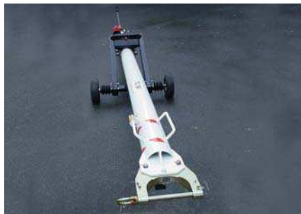
Towbar fitted with the adapter-head for an IL76/86 type aircraft.
